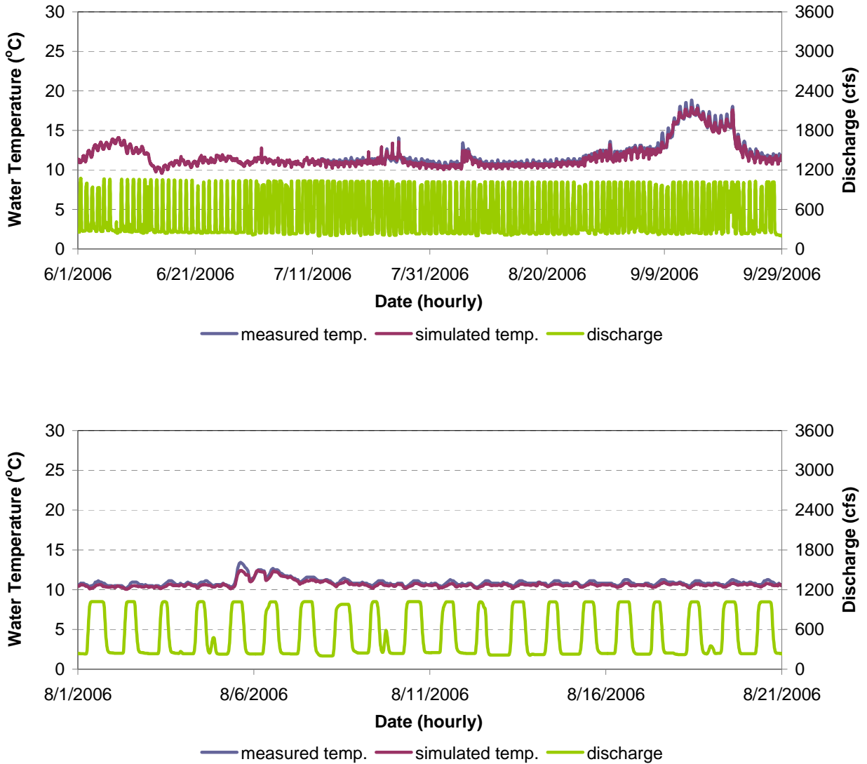
Figure F-35. Water Temperature Model Calibration Results for MF 23.1 in the Ralston Afterbay to Folsom Reservoir Reach of the Middle Fork American River for June 1 - September 30, 2006 (Top) and August 1 - August 21, 2006 (Bottom).
